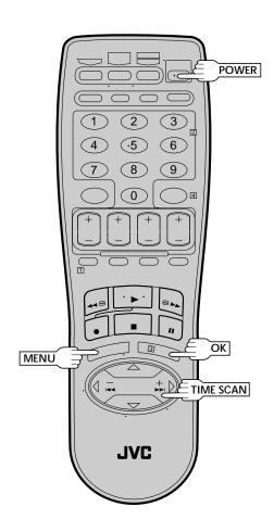
Perform clock setting only if the clock has not been set correctly by the Plug & Play function or you use a cable box. Access the Clock Set screen to perform the Semi-Auto or Manual clock setting procedure. Each procedure starts from step 5. If you use a cable box, set the clock manually. ( pg. 13)
