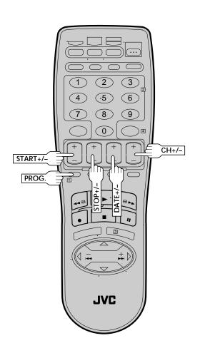
You can directly program the VCR's timer to record up to 8 shows, as far as a year in advance. Remember, the clock must be set before you can program the timer (pg. 8 or 11).
