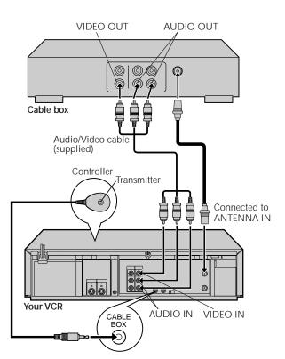
This procedure is required if you receive your TV channels through a cable box (descrambler). The Controller allows the VCR to automatically switch the cable box channel during timer-recording. The Controller is effective for recording shows that have been programmed using VCR Plus+ ( pg. 45) or Express Timer Programming ( pq. 49).
