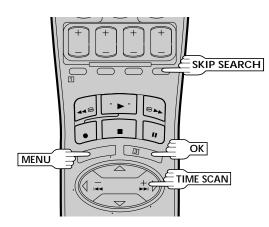
"CA(Commercial Advance) RECORD" and "CA PLAYBACK" are set to "OFF" at the factory. To set Commercial Advance perform the following steps to set "CA RECORD" to "ON" and "CA PLAYBACK" to "AUTO".
