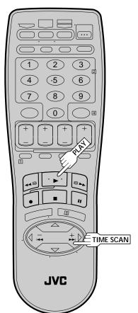
Your VCR is equipped with the TimeScan function. TimeScan allows noise free pictures to be displayed on your TV screen in the forward and reverse search modes. Audio will be played back at normal speed during any of the TimeScan modes (F) pg. 35). TimeScan allows you to view a program in search mode while listening to the audio.
